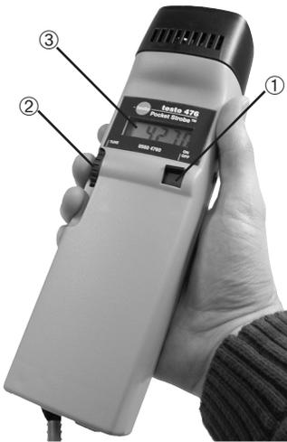
The **testo 476** can be operated with and without mains unit. The Lithium ion rechargeable battery is recharged when the instrument is connected to the mains unit.
