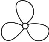
Suppose you want to determine the true RPM of this fan. The only thing you know is that its speed is less than 3,500 RPM. If you slowly decrease the flash rate starting from 3,500 FPM, the following “frozen” images appear:
