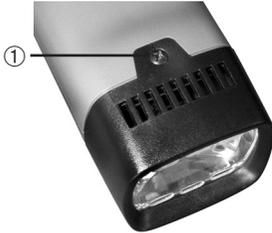
**E1:** Front bezel is not fastened correctly. If the E1 message appears, the instrument must be switched off. Remove the front bezel screw, reset the reflector and tighten the front bezel screw (①).
