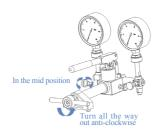
Record 0bar record and close the relieve valve. Providing pressure about 4 bar by hand pump up and down,then adjust the F-adjust valve to second calibration point(5bar).
