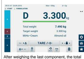
After weighing the last component, the total weight and individual weights of the components can be printed out by connecting an optional printer (depending on the setting in the menu either automatically or after
