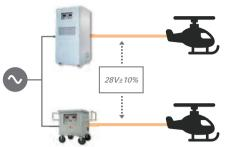
ADS provides stable DC power and has 300% overload capability, which is an ideal ground power solution for the aircraft production and maintenance related industries.
