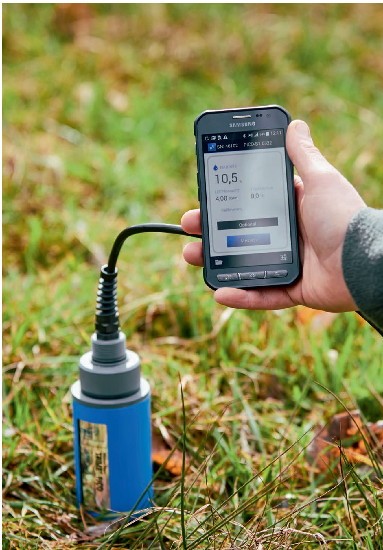
Wireless transmission of measurement data, automatic storage of individual values and calculation of mean values
