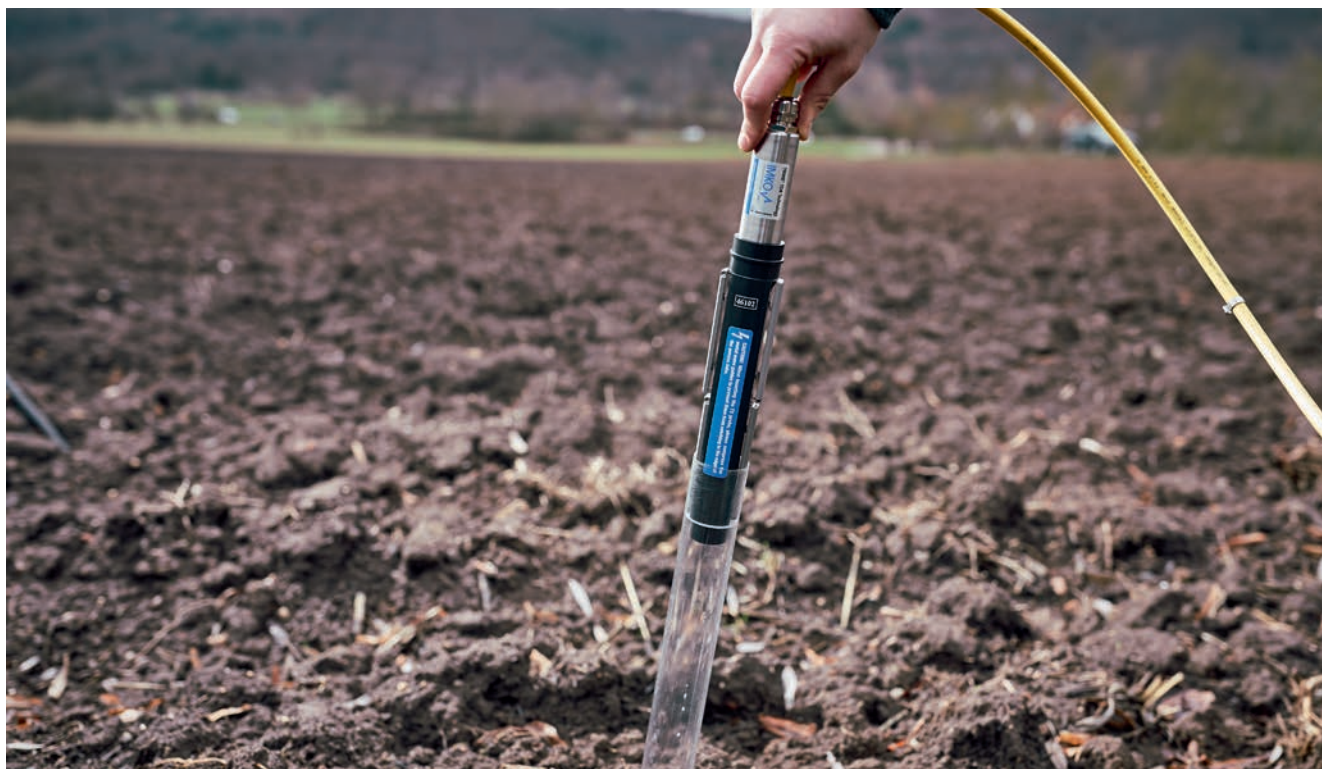
Measuring with the PICO IPH2 using a pre-installed special polycarbonate tube
