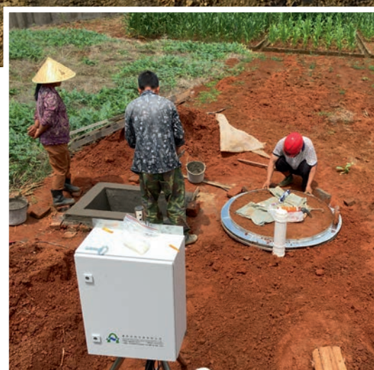
Static installation of PICO probes in an 8m deep lysimeter system in China (in operation, during installation, during the installation of the towers)
