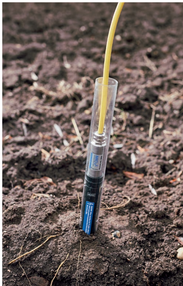
Example of the utilization of an IPH2 in the undisturbed subsoil - the special polycarbonate tube is displayed in the center
