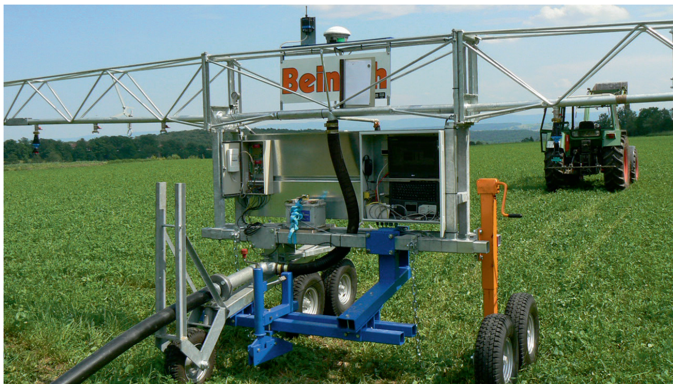
Soil moisture detection by IMKO while field passage of an irrigation cart
