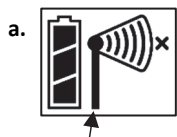
This signal strength icon blinks while searching for a network.
