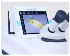
• Integrated CCD camera make it possible save photos /videos for welding result and process for later analysis.
