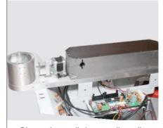
Die cast laser rail give overall sturdiness and accuracy to laser assembly in turn yield powerful laser shot with great depth and stable right from first shot.
