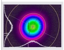
Optical configuration such that it allows to have even energy spot which help better surface finishing of welds and better distribution of filler material.
