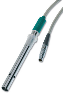
Figure 9: Stainless-steel measuring cell with integrated Pt1000 temperature sensor ( c = 0.1 \text{ cm}^{-1} )
