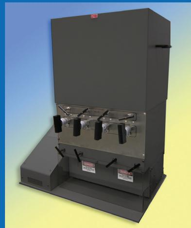
The SFT-120 and SFT-120XW Supercritical Fluid Extractors (SFE) are entry level systems which possess many features typically found in more costly SFE equipment. They may be used for a variety of applications from basic research to process development.
