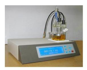
Using Columetrico method to determine trace moisture content of solid, liquid and gaseous.
