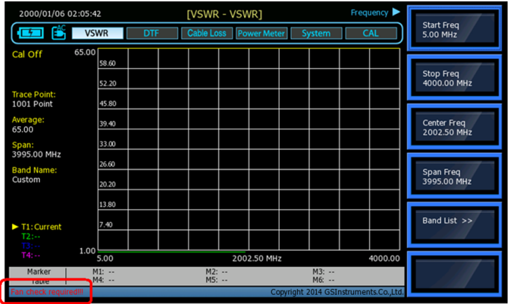
Figure 2.7 FAN Alarm Screen Display
