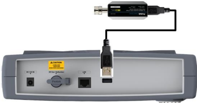
Figure 4.17 Power Sensor Connection Diagram
