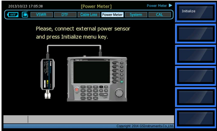
Figure 4.16 Power Measurement Screen
