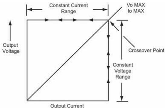
**Figure 4 - CC/CV Characteristic**
