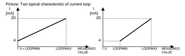
Attention!!! - if measured unit is changed by user, then Loop min value is reset to zero! If value of measured unit is lesser than minimum value, then current of loop is 3,75mA.
