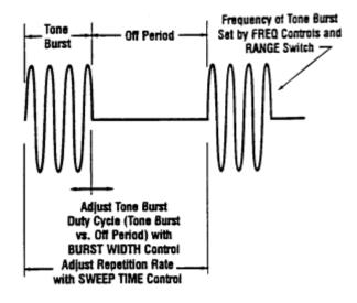
Figure 5. Tone burst generator output waveform.
