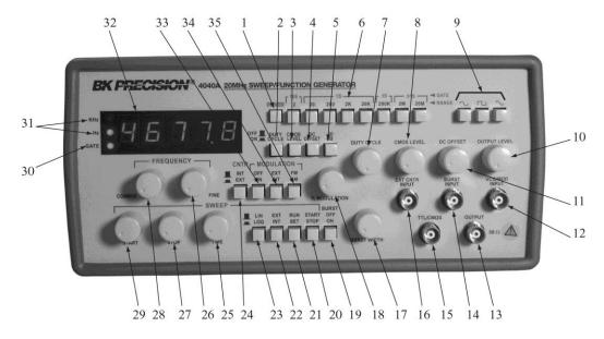
Figure 1. Model 4040A Front Panel.
