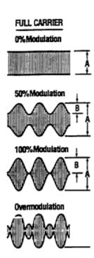
Figure 6. Examples of AM modulation
