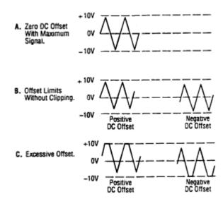
Figure 3. Use of DC OFFSET Control
