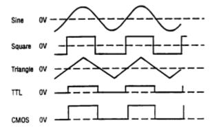
Figure 2. Output Waveform and Phase Relationship
