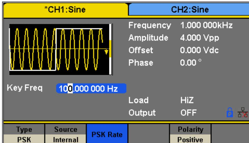
Figure 34 - Setting Interface of PSK Modulation
