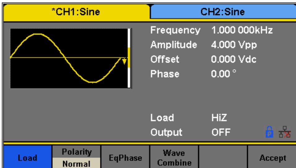
Figure 57 - Output Setup
