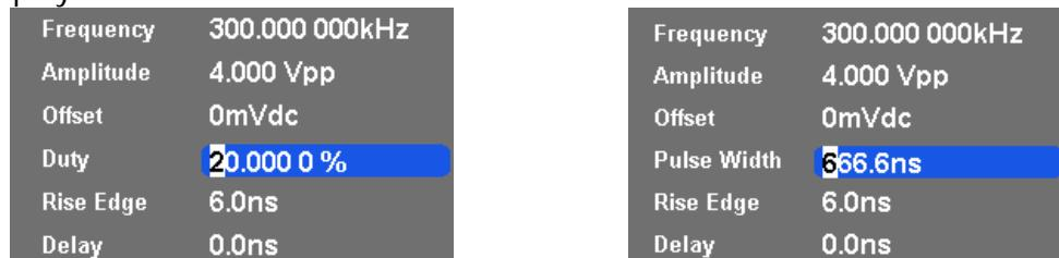
Figure 13 - Pulse Width or Duty Cycle
