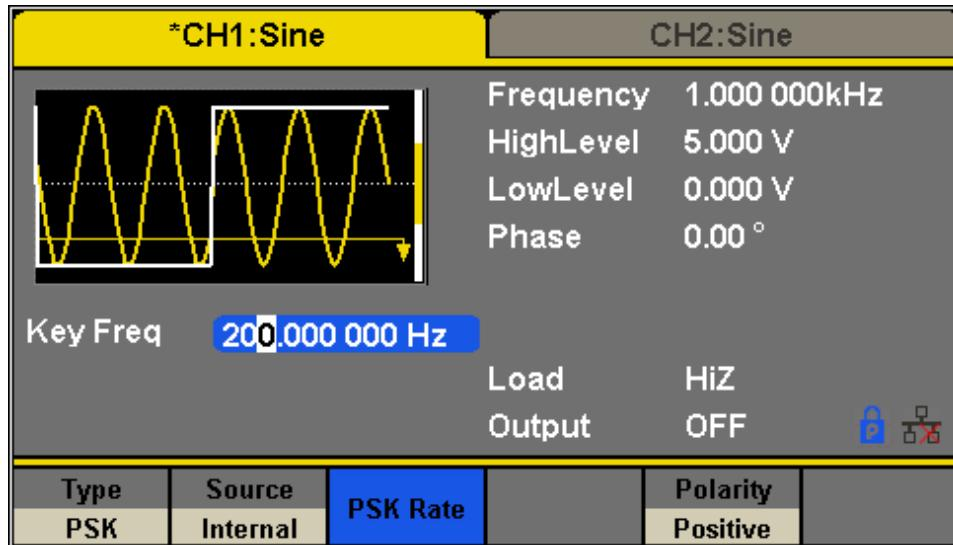
Figure 82 - Generate a PSK Modulation Waveform
