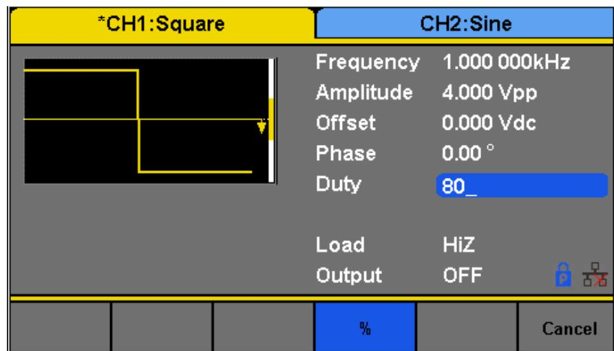
Figure 11 - Duty Cycle of a Square Waveform
