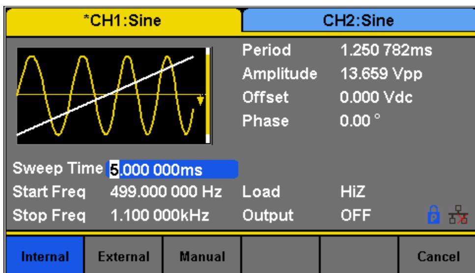
Figure 39 - Trigger Types
