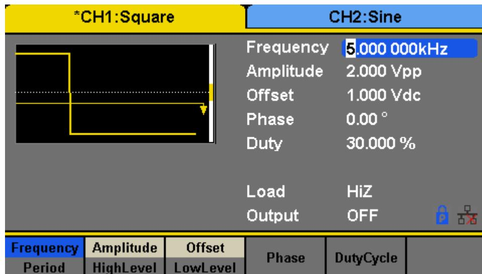
Figure 70 - Generate a Square Waveform
