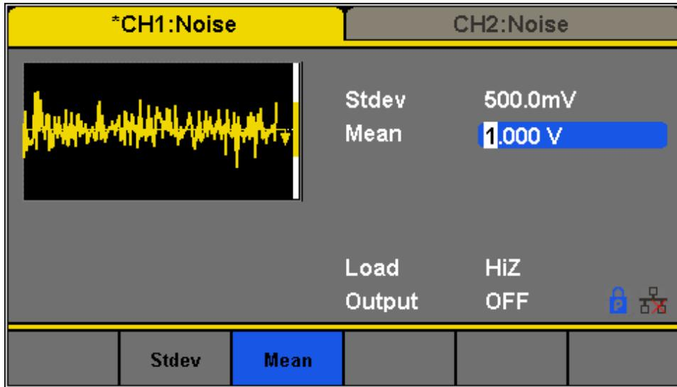
Figure 73 - Generate a Noise Waveform
