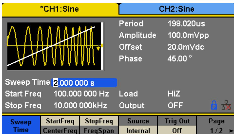
Figure 75 - Generate a Linear Sweep Waveform
