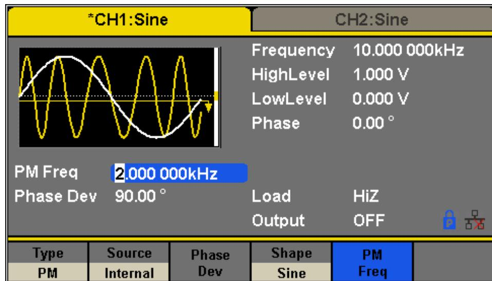
Figure 79 - Generate a PM Modulation Waveform
