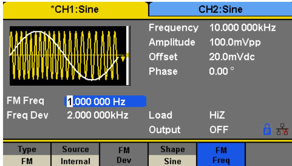
Figure 78 - Generate a FM Modulation Waveform
