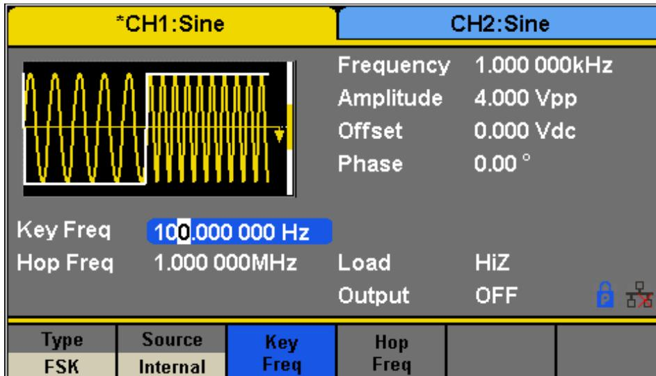
Figure 32 - Setting Interface of FSK Modulation
