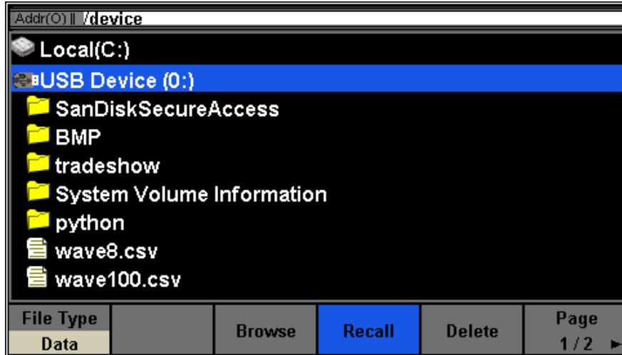
Figure 26- Load an Arb Waveform from External
