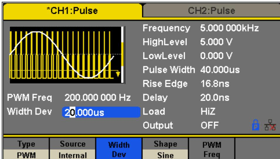
Figure 83 - Generate a PWM Waveform
