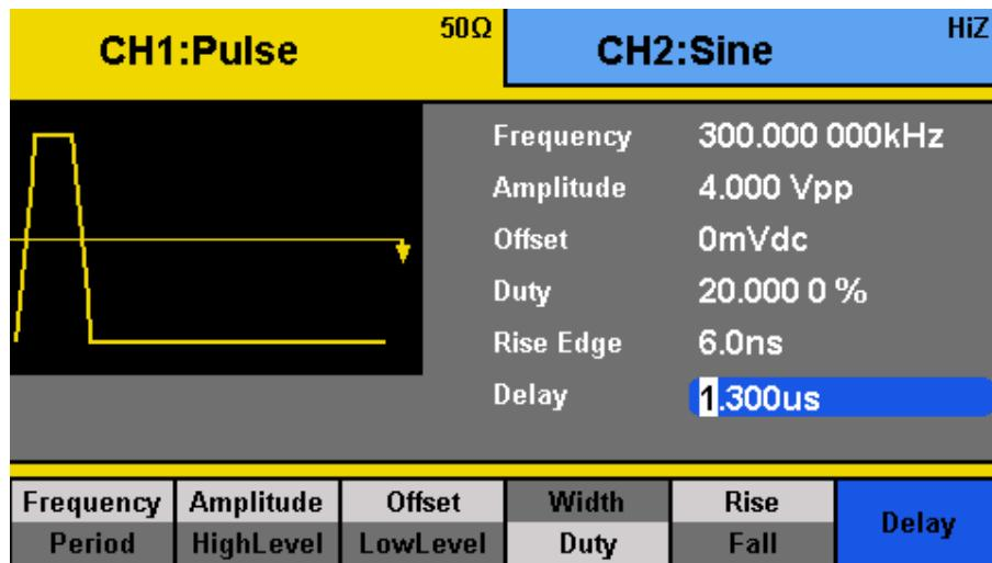
Figure 16 - Pulse Delay
