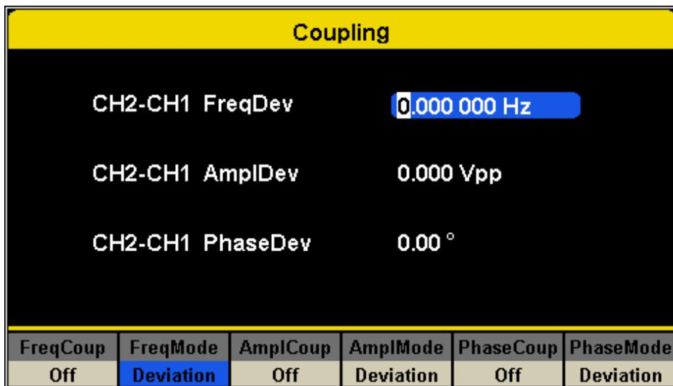
Figure 60 - Channel Coupling
