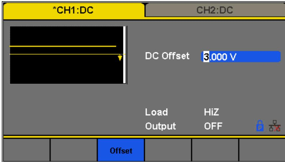
Figure 74 - Generate a DC Waveform
