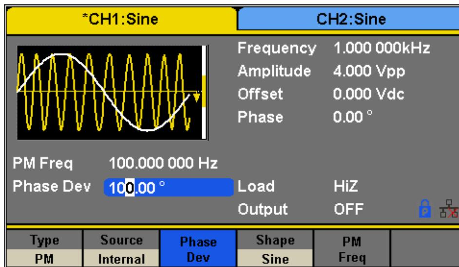
Figure 31 - Setting Interface of PM Modulation
