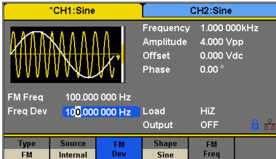
Figure 30 - Setting Interface of FM Modulation
