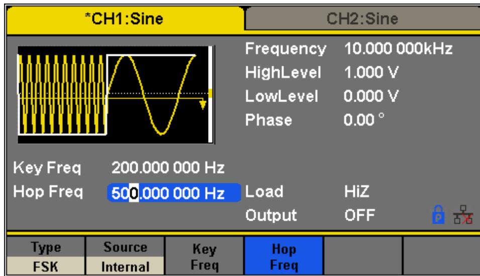
Figure 80 - Generate a FSK Modulation Waveform
