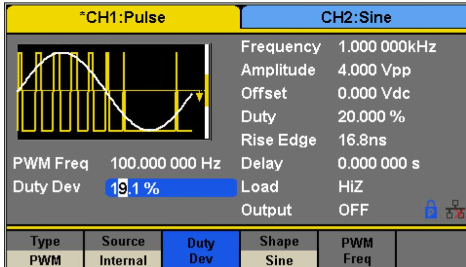
Figure 35 - Setting Interface of PWM Modulation
