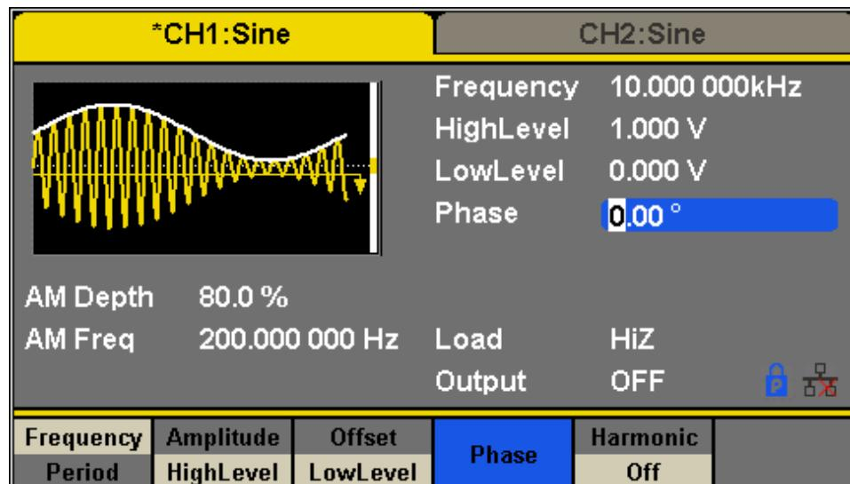
Figure 77 - Generate an AM Modulation Waveform
