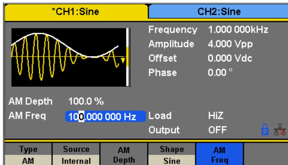
Figure 28 - Setting Interface of AM Modulation
