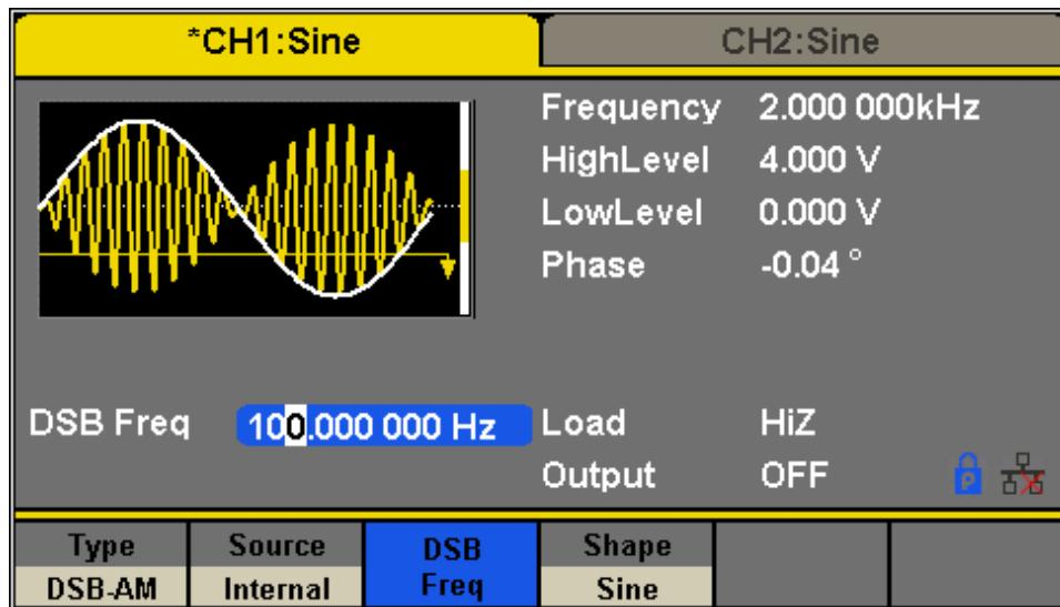
Figure 84 - Generate a DSB-AM Modulation Waveform
