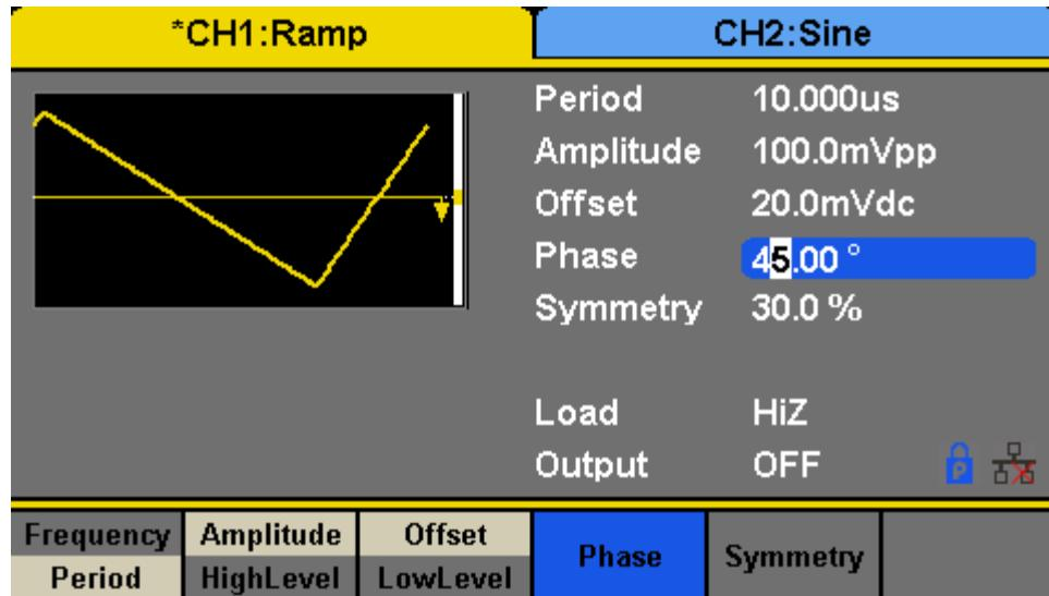
Figure 71 - Generate a Ramp Waveform
