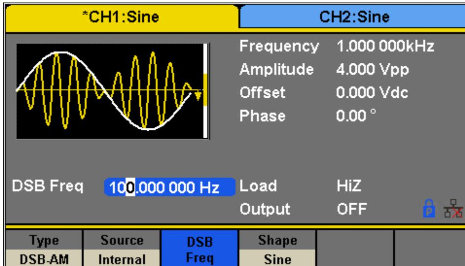
Figure 29 - Setting Interface of DSB-AM Modulation
