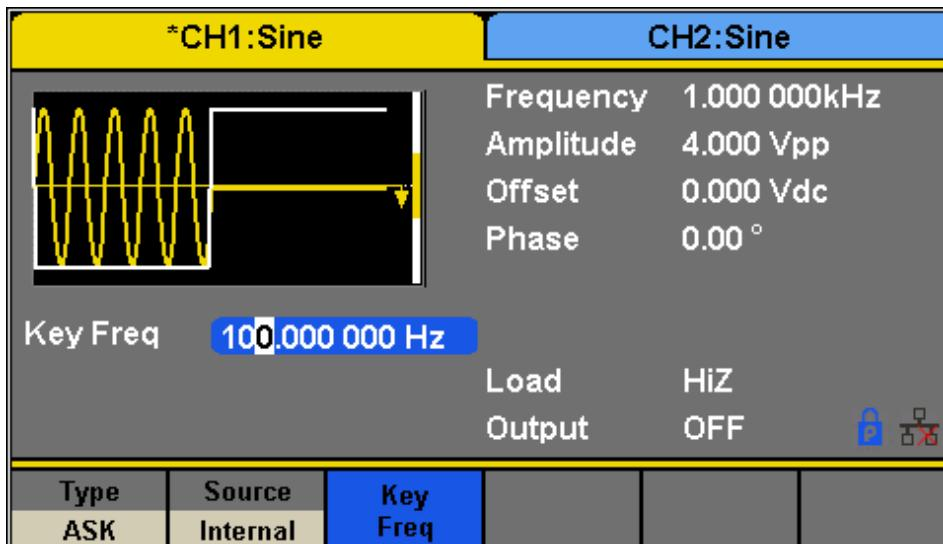
Figure 33 - Setting Interface of ASK Modulation
