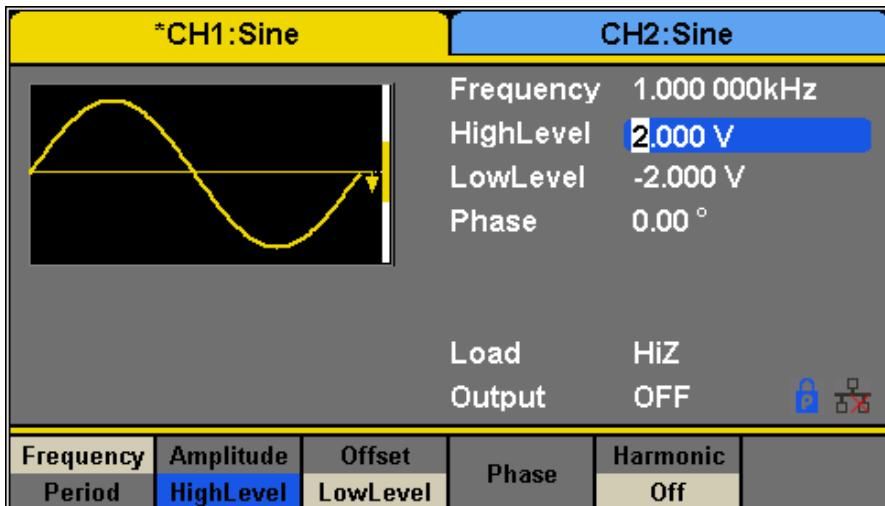
Figure 7 - Amplitude: High and Low Level
