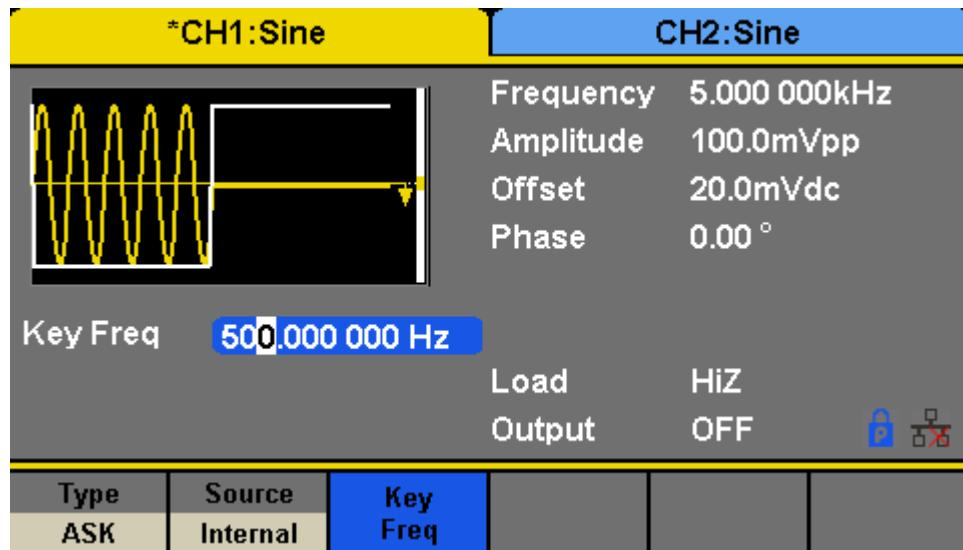
Figure 81 - Generate a ASK Modulation Waveform
