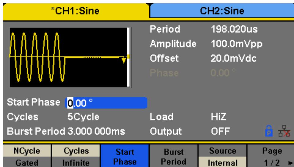
Figure 76 - Generate a N-Cycle Burst Waveform
