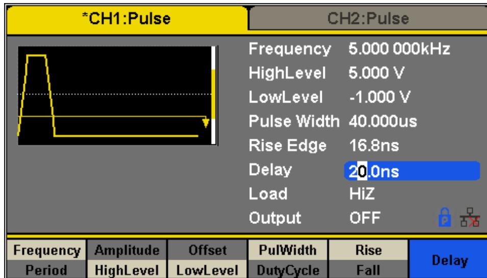
Figure 72 - Generate a Pulse Waveform
