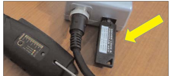
To adjust the settings the Program Lock Key must be plugged into the STC40 & FT-30D Mini Transformer.
