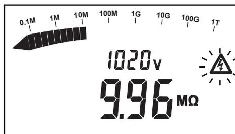
During measurements the instrument will beep every 10 seconds to alert the user that a high voltage is present.
