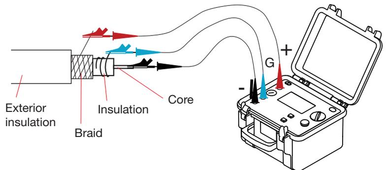
The guard serves to eliminate the effect of surface leakage currents.
