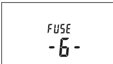
Indicates that the protective fuse of the G terminal is defective.
