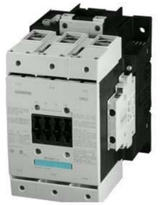
CONTACTOR, 55KW/400V/AC-3 AC(40...60HZ)/DC OPERATION UC 21...27,3V AUXIL. CONTACTS 2NO+2NC 3-POLE, SIZE S6 WITH BOX TERMINALS ELECTRONIC OPERATING MECHANISM WITH PLC INTERFACE 24V DC SCREW TERMINAL
