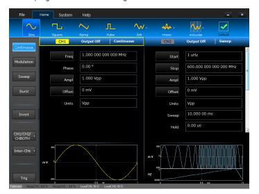
In Advanced mode, users can define complex waveforms with up to 16,384 entries of analog waveforms and digital patterns in a sequence, in terms of loops, jumps, and conditional branches.
