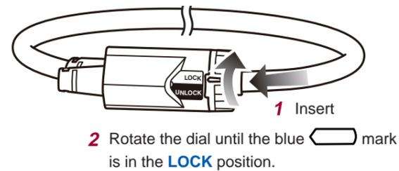
Pulling on the flexible loop with a large amount of force while in the locked state may cause it to become disconnected from the coupling.
