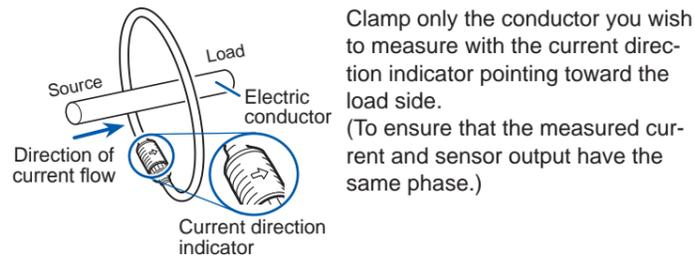
Clamp only the conductor you wish to measure with the current direction indicator pointing toward the load side. (To ensure that the measured current and sensor output have the same phase.)
