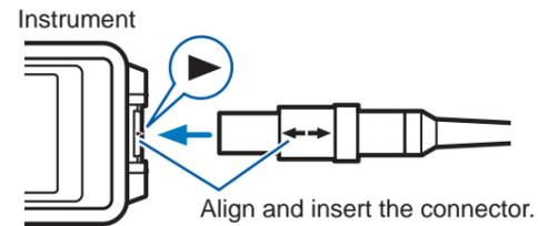
Align the arrow on the device's output connector with the ► on the connected instrument's sensor input connector and insert the connector.
