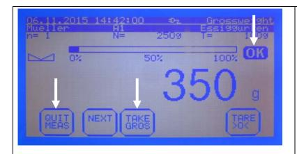
After the first measurement object has been placed it will be confirmed with TAKE GROS. The balance jumps automatically to the second target.
