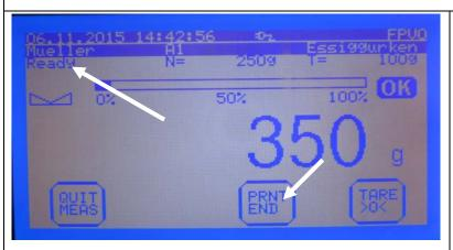
After the last measurement object the scale displays "Ready" and the series of measurements can be printed with PRNT END.
