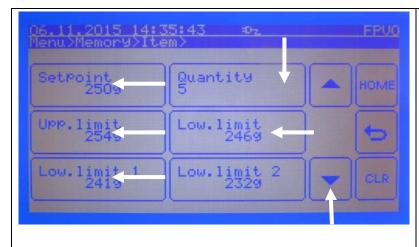
Here, the tolerance data as setpoint, upper limit, lower limit, lower limit 1 and lower limit 2 can be entered.
