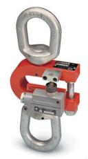
The heart of the system is a force beam which operates in tension or compression. Seven different load capacities are available. Switch and physical connection options are listed. Each beam can accommodate from one to four switches which can be set to operate as many as four different switching functions or combinations including slackline detection.
