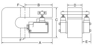
25,000 lb and 50,000 lb capacity force beam. Illustrated above two weatherproof switches (option 2B).
