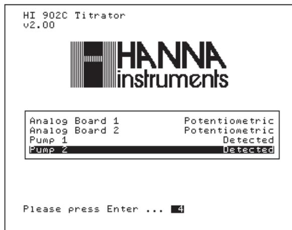
**Note:** All the performed initialization processes must be successfully completed. If one of them is terminated by a "Failed" message, restart the titrator from the power switch. If the problem persists, contact your dealer.
