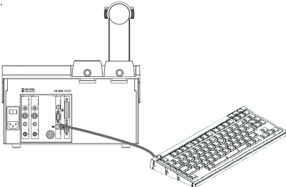
Connect an external PC Keyboard (PS/2 connector).
