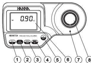
1. GLP/▲ key: press to enter *GLP mode*. In *calibration mode* press to edit the date and time.
