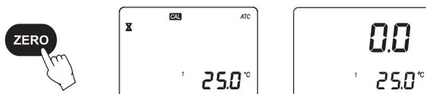
**Note:** The 0.0 screen will remain until a sample is measured or the instrument is turned off.
