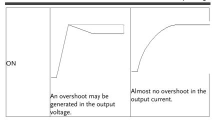
The above voltage and current waveforms assume that the resistance is the load of this unit.
