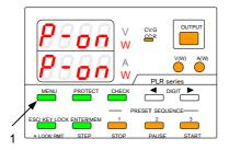
2. The output setting for when the power is turned on must be set to "on" by using the MENU key and rotary encoder.
