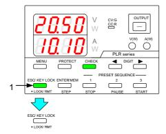
Even if the unit is in local mode, it returns to remote mode when it is operated via external digital control.
