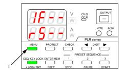
If the mounted interface card is the PLR-GU, PLR-LU, or PLR-RS (all of which allow the unit to be controlled remotely), the system address and PC address can be displayed by pressing the MENU key while "IF--" is displayed.
