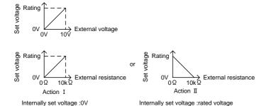
Set voltage control via external signal (Valid when pin No.4 of SW1 is on)
