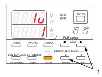
2. While the STOP key is lit in amber (while the sequence program is stopped), press the DIGIT key ◀ to pause the sequence at the last step.
