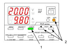
3. Press the DIGIT ◀ ▶ keys to move the blinking digit in the current indicator.
