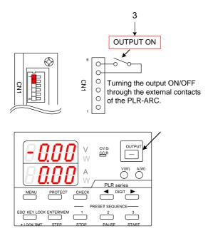
4. Use the external contacts of the PLR-ARC board to turn the output off.
