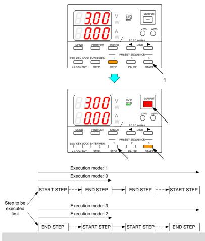
Automatic execution cannot start from a step that is in the middle of the sequence program.
