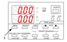
Press the DIGIT keys ◀ ► to select the digit to be modified. Only the digit that is blinking can be modified.
