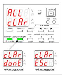
(2) Clearing the setting data for manual operation
