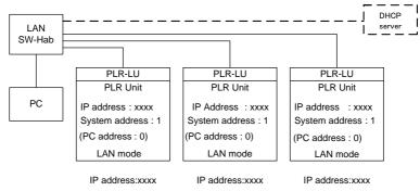
The LAN uses an XPort (manufactured by Lantronix) that supports Ethernet (IEEE 802.3) communication. A RJ45 connector (10BASE-T or 100BASE-TX) is used to connect the Ethernet interface.
