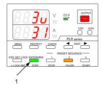
The figure on the left indicates that the program is in the 3rd execution cycle, from the start step to the end step, and that step 31 is being executed.
