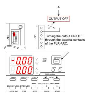
In the PLR power supply unit, when the output of the unit has been turned on through the external contacts of the PLR-ARC board, the OUTPUT key on the front panel can be used to turn the output on or off during operation.
