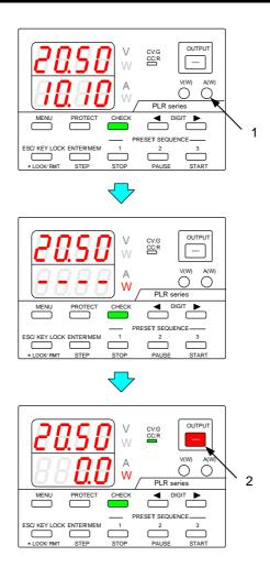
When the V and A keys are lit, the display cannot be switched to the output power display.
