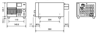
• 720W model : Outside dimensions: 124mm (H)  $\times$  210 mm (W)  $\times$  364mm (D) Weight: Approx. 7.5kg
