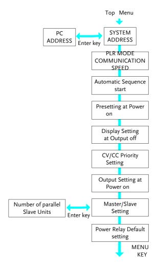
The following items can be set when turning on the power switch while pressing and holding the ENTER/MEM key:
