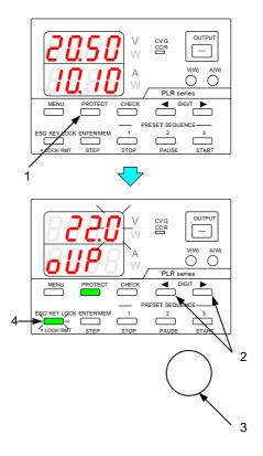
Press the green-lit PROTECT key to change the display. The display changes in the following order: OVP setting  $\rightarrow$  UVP setting  $\rightarrow$  OCP setting.
