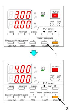
While a sequence program is paused, only the step execution time is paused. The other step setting items continue being executed. If the output is set to be on for the step being executed, the unit output will be on.
