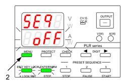
3. Turn the rotary encoder to display "on" in the current indicator.
