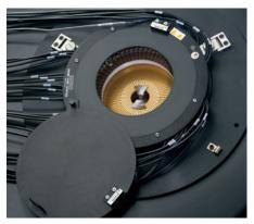
The Model 9139A Probe Card Adapter has been trusted by the industry for more than 10 years. Its combination of low current performance and high voltage capability makes it the ideal companion to the S530 Parametric Test Systems.
