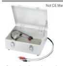
This is used as a sample accommodation box during measurement of a high-insulation resistance samples, or inductive or capacitive samples to perform electromagnetic shielding.
