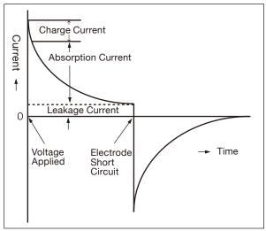
Absorption Current Characteristic Curve
