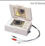
Not CE Marked Sample of 100mm square by up to 8mm in thickness is measurable. The main electrode dia. is 50mm and inner & outer dia. of ring electrode are 70mm & 80mm respectively. Measurement voltage becomes "OFF" while the lid is open to ensure safety. A selector switch allows selection of voltage or surface resistivity.
