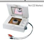
Sample of 40~100mm square by up to 8mm in thickness is measurable. The main electrode dia is 19.6mm and inner & outer dia. of ring electrode are 24.1mm & 28.8mm respectively. Measurement voltage becomes "OFF" while the lid is open to ensure safety.
