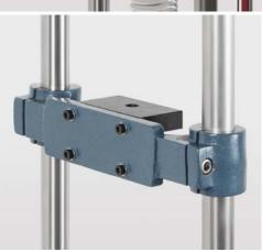
The external force measuring cell hast tob e mounted at the fitting bracket AFM 41 with a M12x40 screw (at TVM 5KN and 10KN) and with a M12x80 screw (at TVM20KN and TVM 30KN), included in delivery.
