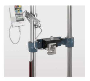
The FH force gauge mounted on the test stand now has to be connected by means of the RS232 cable with the test stand to the Equipment-Port.
