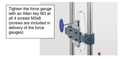
Force gauge with internal force cell mounting, finished:
