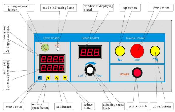
**Power key:** controls the whole machine's power, on and off.
