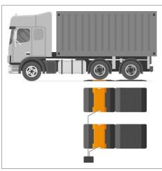
Asynchronous weighing of double axles which are installed next to each other, using compensation pads
