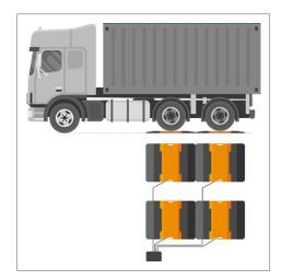
Simultaneous weighing of double axles, e.g. of a trailer
