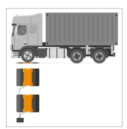
**Asynchronous weighing of individal axles**Order example: standard package VHP 6T-3
