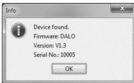
Fig. 4: Software response after positive test connection to DALO, in the example with serial number 10005 and for firmware version 1.3.
