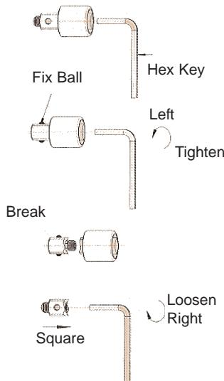
The break-away safety adapter is inserted into the square opening of the torque multiplier.
