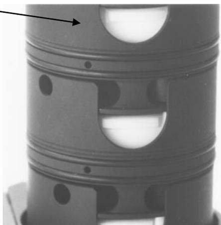
**Attention:** Don't scratch or damage the black coatings of all internal pieces. Failures can have influence regarding the photometer measurement.
