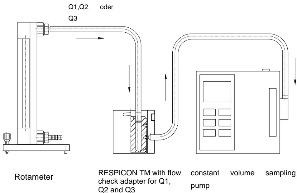
The total flow rate,  $Q_G$ , can also be measured directly. Remove the fitting from the flow checker and put the tube adapter (part #: 001.0085.005) on the flow checker. Make sure that there are no leaks.
