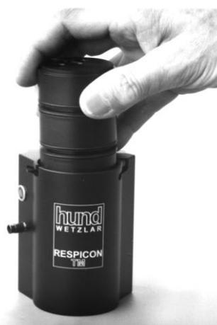
Press it completely into the mantle. Eventually use the inlet head or the tube adapter.
