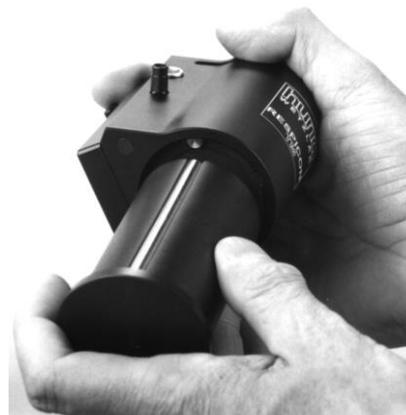
Put the disk on the sampling instrument.
