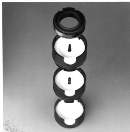
Before starting the sampling procedure assemble the filter supports loaded with cassettes and filters as follows: put support #2 on top of support #3, and support #1 on top of support #2. The ring labels of the supports must be at the top.
