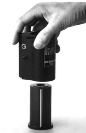
Put the flat disk on the sampling instrument. Press steadily on the disk. The filter supports will come loose and the mantle can be pushed down.
