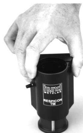
Stack up the filter supports loaded with cassettes and filters on the assembling cylinder. Make sure that they are in the right order, i.e. #3 at the bottom, #1 at the top.
