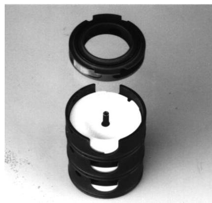
Now put the mantle of the instrument over the assembling cylinder.
