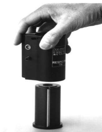
The pin on the underside of the body unit must be put into the corresponding groove of the assembling cylinder.
