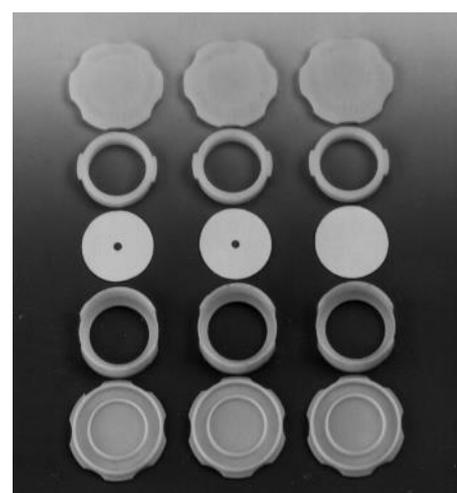
Insert the filter in the cassettes (part number: 001.0001.017). Then put the filter cassettes containing the filters with hole into the supports #1 and #2, respectively, and put the filter cassette containing the filter without hole into the support #3.
