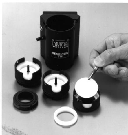
Each of the filter support units is labeled by one or several carved rings on the upper section of its mantle.
