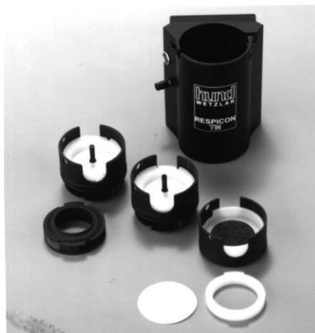
The filters must be carefully centered in relation to the filter-cassettes and filter - supports no. 1 and no. 2. For that reason first insert the filter-cassettes into the filter-supports. Than insert (center) the filter to the filter-cassettes and lock each filter-cassette with the top ring (coverlid) of the filtercassette.
