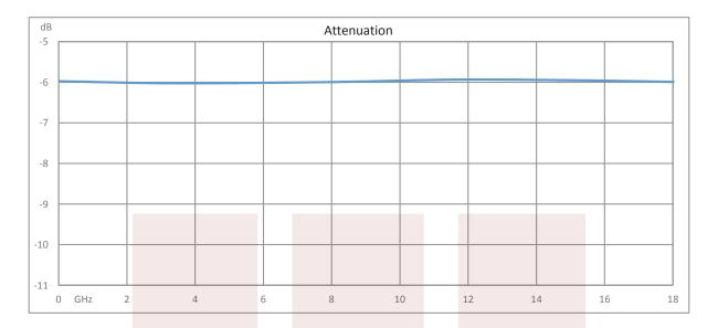
6 dB Fixed Attenuator SMA Male To SMA Female Up To 18 GHz Rated To 2 Watts With Passivated Stainless Steel Body from Fairview Microwave is in-stock and available to ship same-day. All of our RF/microwave products are available off-the-shelf from our ISO 9001:2008 certified facilities in Allen, Texas. Fairview Microwave is RF on-demand.
