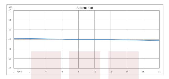
13 dB Fixed Attenuator SMA Male To SMA Female Up To 18 GHz Rated To 2 Watts With Passivated Stainless Steel Body from Fairview Microwave is in-stock and available to ship same-day. All of our RF/microwave products are available off-the-shelf from our ISO 9001:2008 certified facilities in Allen, Texas. Fairview Microwave is RF on-demand.
