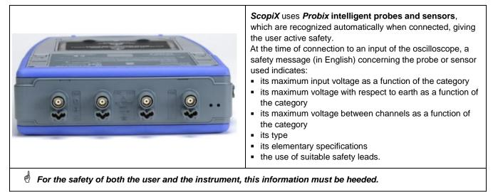
The trace colour of the signal measured with a given accessory is parameterized in the menu: "Green"  $\rightarrow$  "chX"  $\rightarrow$  "Probix". An interchangeable elastic or plastic ring is used to associate the colour of the probe and the colour of the curve. Scaling and units are managed automatically by the **Probix** system, allowing rapid measurements with no risk of error.
