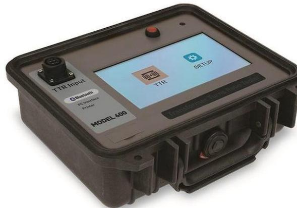
TEKON600 is a test set that measures the turns ratio of windings in single phase distribution with the application of 7" wide touchscreen aimed to maximize user convenience. In particular, it can be used anywhere as it is powered by chargeable battery. Selectable test voltages include 4Vac, 10Vac, 40Vac and 100Vac (optional), enabling you to measure a variety of transformers.
