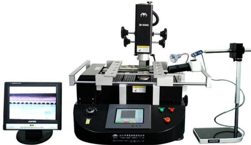
1. Adopt liner slide which makes X, Y, Z axis all can do high positioning accuracy and fast maneuverability.
