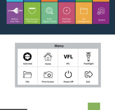
Press the "Shortcut menu" icon to enter the quick operation menu, and press different function icons to enter the corresponding function interface or realize the corresponding operation function.
