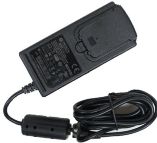
Fig. 1: Power supply unit 5 V DC/4 A in accordance with EN 61558-2-16, DC socket 2.1 mm, SK-II, 12651-99
