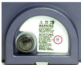
Fig. 5: Screw holding the cover
