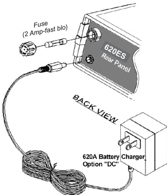
A fully charged battery pack typically powers the 620ES for approximately 6 ~ 8 hours before requiring a recharge. AMPTEC installs a quality set of 4 each Heavy Duty (5000 mAhr) Ni-Cad batteries. The 620ES will also operate on a 4000 mAhr D cell Ni-Cads with a shortened operating time between charges. Recharge time is typically twice the “Power On” time. An “Overnight” charge usually restores the 620ES to a “Fully Charged” ready to use state.
