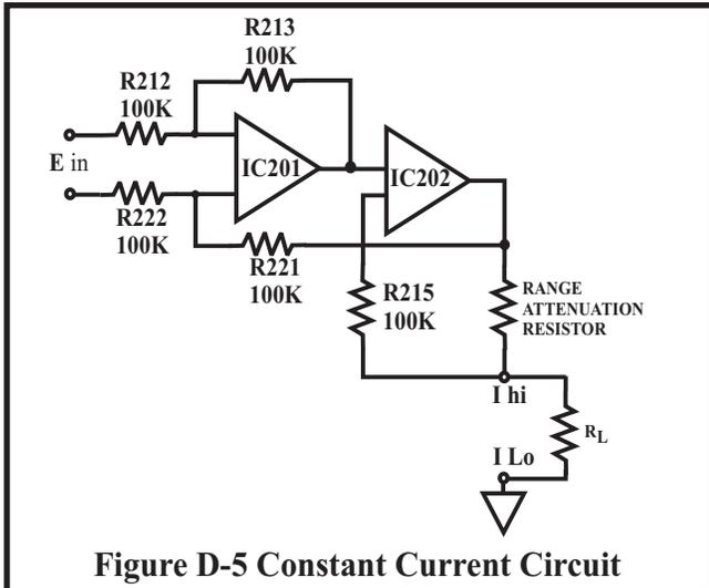
Figure D-5 Constant Current Circuit
