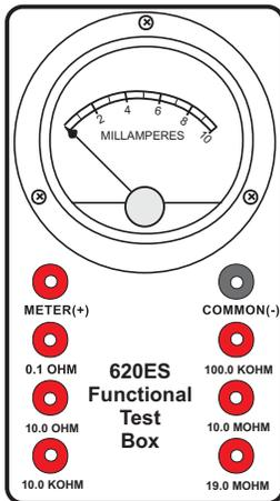
**Functional Test Section** - The optional 620ES Functional Test Box provides added measurement integrity using a milliammeter and test resistors to cross check the overall 620ES operation whenever desired. The test resistors are for cross checking 620ES basic operation and should not be used for calibration purposes.
