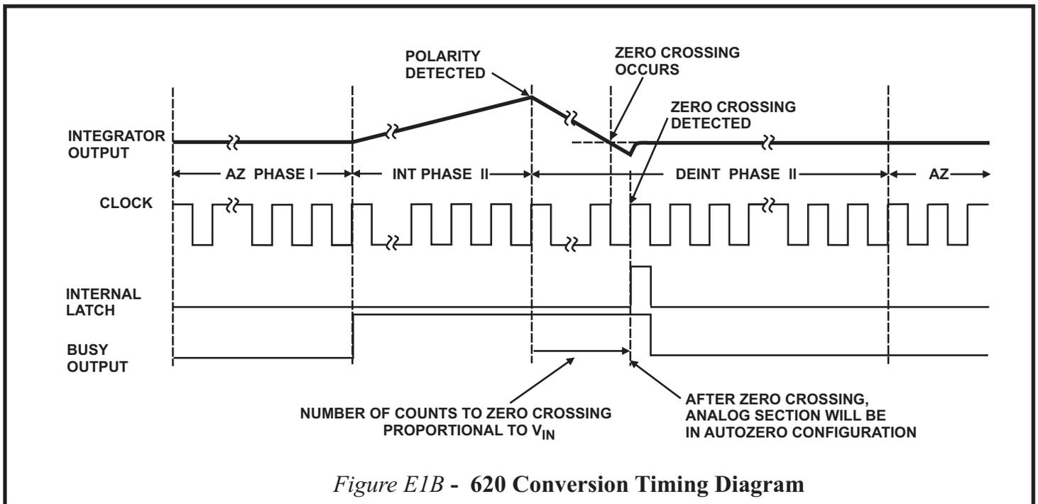
Figure E1B - 620 Conversion Timing Diagram
