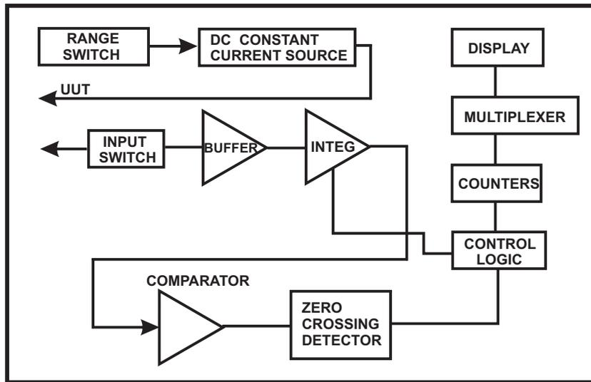
Figure E1 - AMPTEC 620ES FUNCTIONAL BLOCK DIAGRAM
