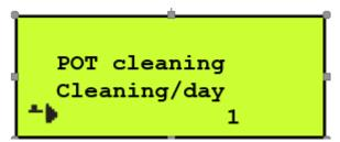
Note: When set to 0, the cleaning feature is deactivated. A maximum 4 cleaning processes can be carried out per day. The start of the cleaning is controlled by the internal clock. The first cleaning/day will be carried out at 0:00.
