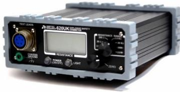
The AMPTEC 620UK Safety Ohmmeter is a portable EEX digital ohmmeter for ultra-safe resistance testing in explosive and volatile atmospheres. The 620UK's ultra-safe design allows it to comply with the EU ATEX Directive, the Intrinsic Safety Standard Eex-9b-IIC-T4, and USA MIL STD 810 as well as many other international defense standards. For testing of squibs or explosive bridge-wire, the AMPTEC 620UK is a clear choice for munitions experts both domestically and internationally.
