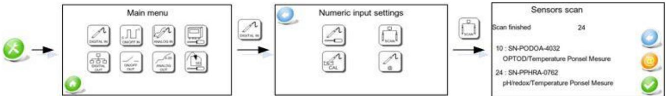
As soon as the transmitter detects a sensor, it displays its address, its serial number (which is also engraved on the body of the sensor) and a description of the sensor.
