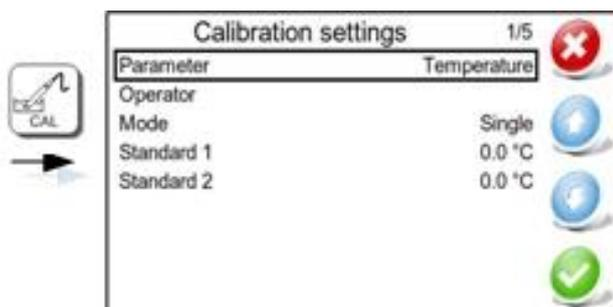
The **Calibration settings** window lets the operator: select the parameter to be calibrated; enter the operator's name; select a calibration mode and set the values of the standards used.
