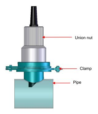
1 After welding the clamp on the stainless steel pipe, remove the clamp from the system and remove the PVC adapter.
