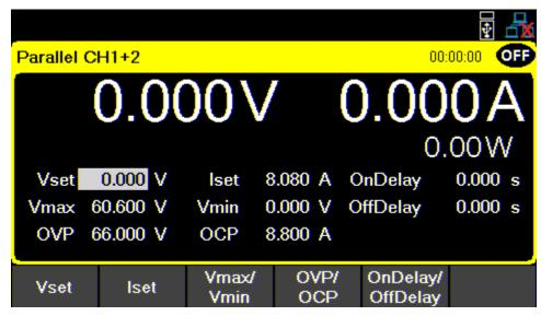
Figure 4.14 Parallel CH 1+2 Single Channel Display
