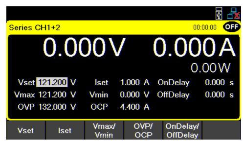
**Figure 4.8** Series CH1+2 Single Channel Display
