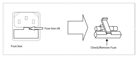
Figure 2.1 Fuse Removal
