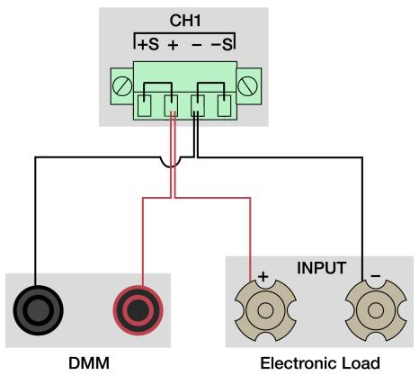
Figure 11.2 Rear Panel Wiring Diagram
