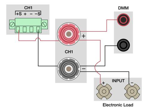
Figure 11.1 Front Panel Wiring Diagram
