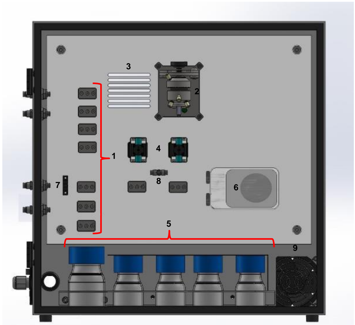
Figure 8 Overview inside BACTcontrol (frontside)
