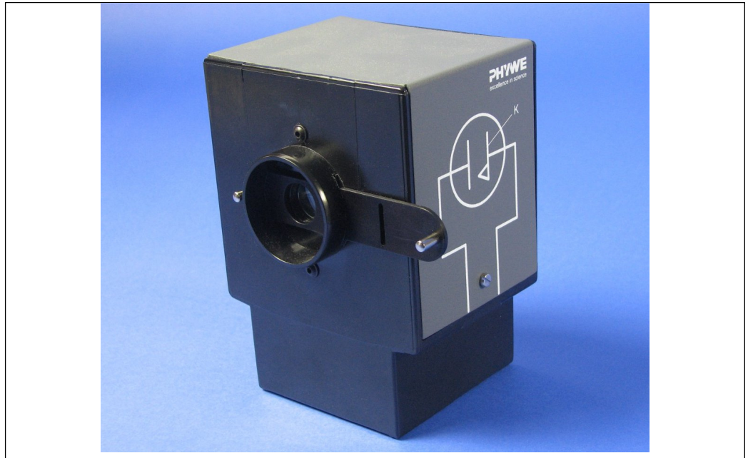
Fig. 1: Photocell for determination of Planck's constant h with housing 06779-00
