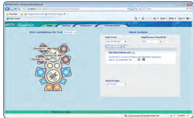
Figure 4 — TOOLweb RGA homepage screen for a tool with Vision 2000 XD degas modules
